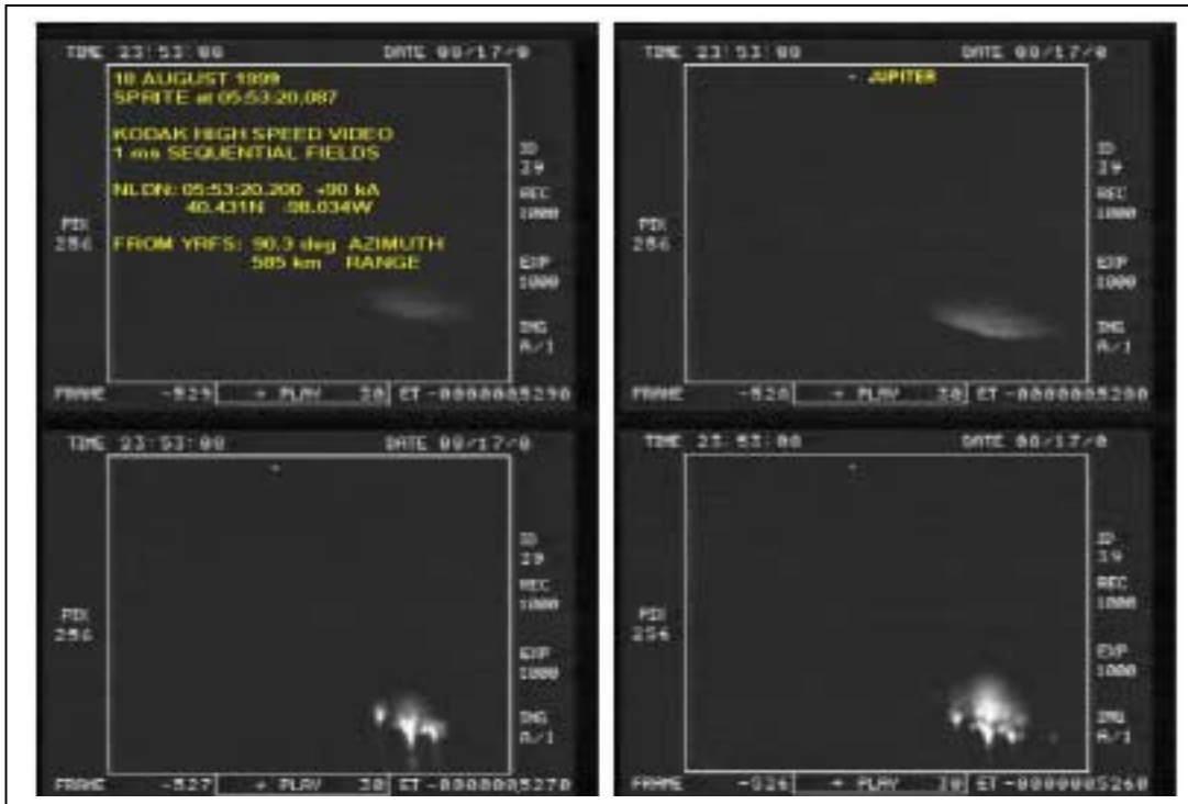
Figure 1. High speed (1000 fps) image intensified camera showing the descending disk of a sprite halo (first two 2 ms) followed by the emergence of sprites from the halo's bottom ledge.
